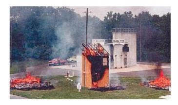
The results of this demonstration correspond closely with the results achieved by the National Fire Laboratory of the National Research Council Canada. The cellulose insulation structure maintained its structural integrity, for a total time of 68.08 minutes, in excess of 24 minutes longer than the fiberglass structure or the uninsulated structure translating to an increased fire resistance of 57% as compared to the 55% improvement achieved in the laboratory study.
